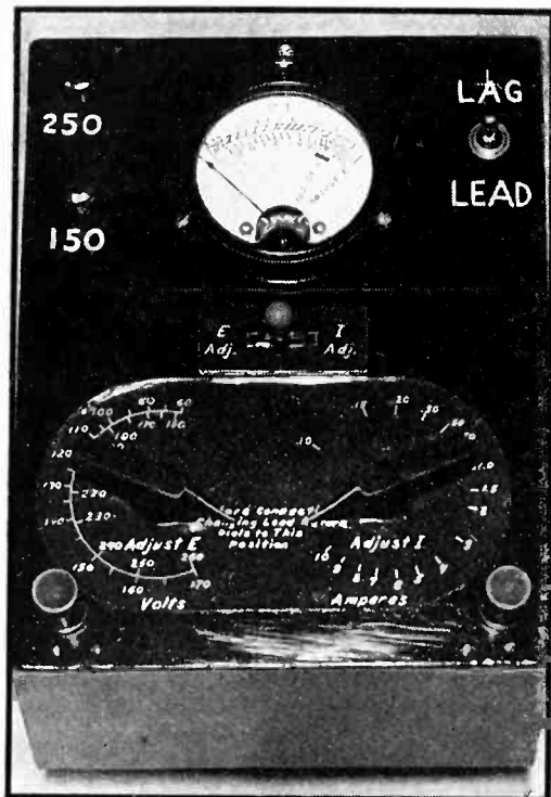
Photograph of the power factor meter which reads leading or lagging power factor directly on 150 or 250 volt circuits
